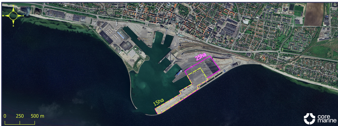
Figure 8 - The relative size needed for storage at the port of Trelleborg. Much of this area is used for other purposes and additional designated areas for offshore wind components would have to be investigated in cooperation with the port owner/operator.
