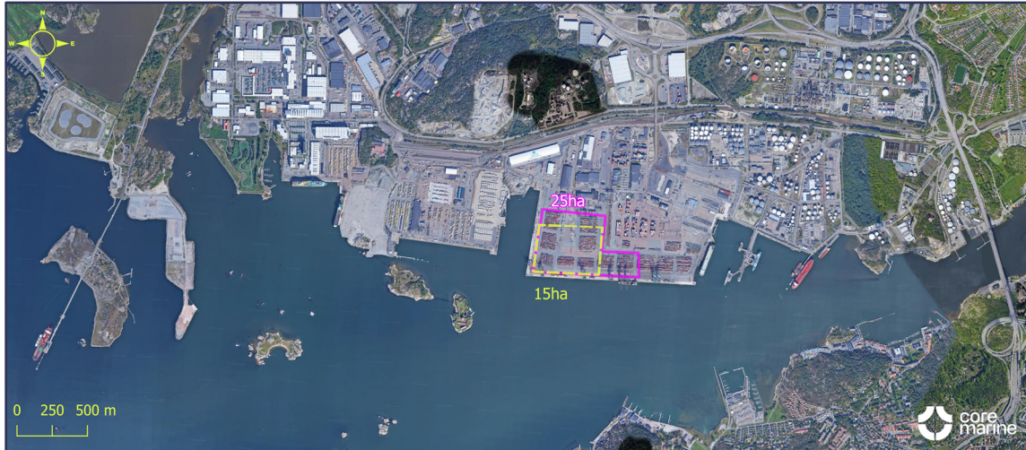
Figure 7 - The relative size needed for storage at the port of Gothenburg. This area is used for containers and designated areas for offshore wind components in the port would have to be investigated in cooperation with the port owner/operator.
