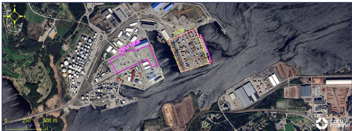
Figure 9 - The relative size needed for storage at the port of Gävle. Much of this area is used for containers and designated areas for offshore wind components would have to be investigated in cooperation with the port owner/operator.
